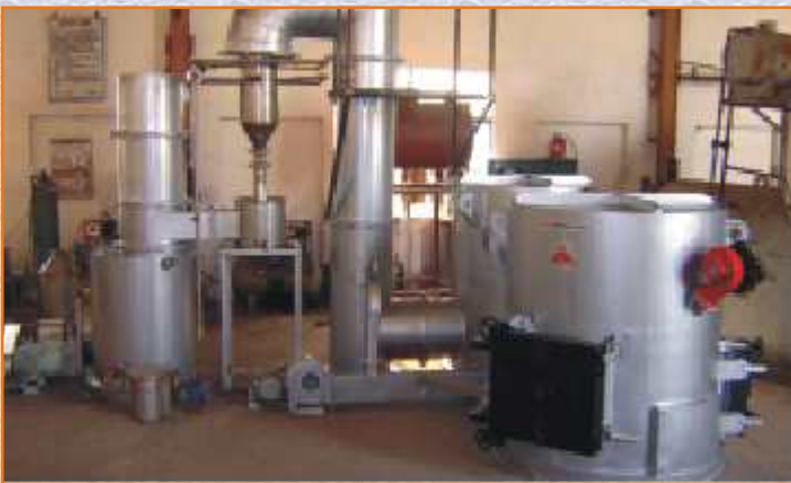
Incinerator with Venturi Scrubber
