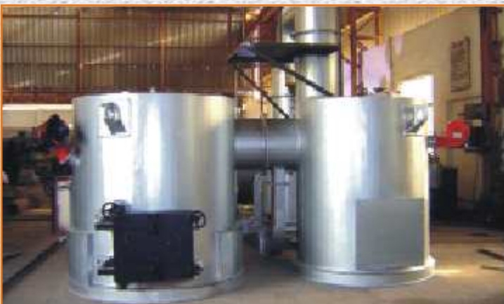
Primary and Secondary Chambers of Horizontal Incinerator
